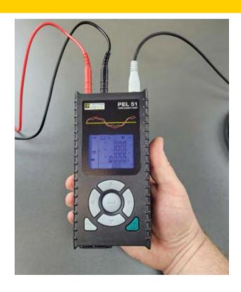
The Electricity Safety, Quality and Continuity Regulations (ESQCR) 2002 state a permitted voltage tolerance of 230 – 6% +10%, and it is the responsibility of the Distribution Network Operator (DNO) to maintain the supply voltage to within these limits. Accordingly, many EV charger manufacturers set a maximum supply voltage threshold of 253 V, however, there are a growing number of EV owners experiencing problems, with mains voltages as high as 259 V being reported.
