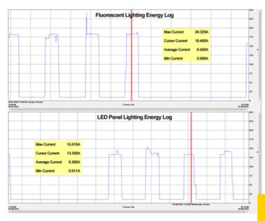
A little maths reveals that with a measured voltage of 243.6V and power factor of 0.905PF, we were consuming 4,058W. Following replacement with LED units the second log showed that this has gone down to 2,943W, essentially reducing our energy use for office lighting by 25%.
