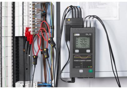
PELs are capable of storing millions of readings, and data can be retrieved locally or remotely via Bluetooth, WiFi, 3G/ GSM, USB or Ethernet. It's even possible to combine a number of PELs together to track several consumption points around a facility or multiple facilities, and without the expense of travel to retrieve the data.
