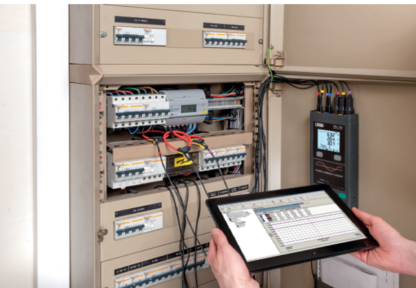
PEL energy logger with tablet for recording aspects of the energy supply.
