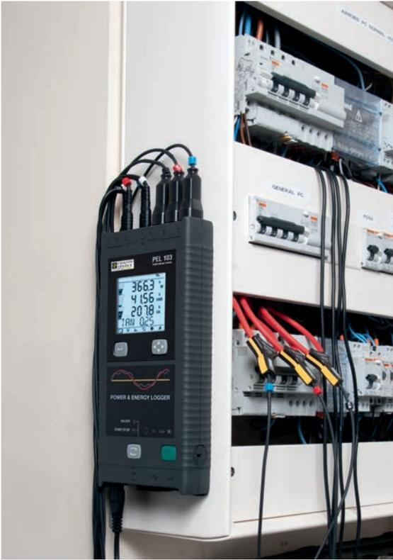
Thankfully, measuring energy consumption, including where and when it is being used, and monitoring other parameters such as power factor and harmonics, has never been easier thanks to portable **Power and Energy Loggers** or **PELs**.
